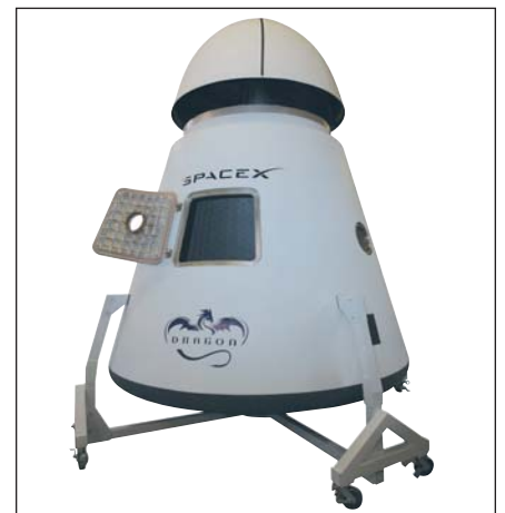
The Dragon spacecraft is made up of a pressurized capsule and unpressurized trunk used for Earth to LEO transport of pressurized cargo, unpressurized cargo, and/or crew members. Image: SpaceX
