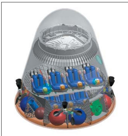
The Dragon spacecraft is made up of a pressurized capsule and unpressurized trunk used for Earth to LEO transport of pressurized cargo, unpressurized cargo, and/or crew members. Image: SpaceX
