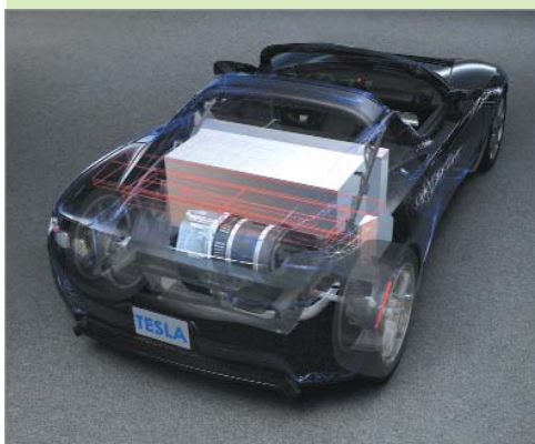
Under the skin of the Roadster is a battery box, air ducts that double as energy-absorbing zones, and a high-performance AC motor.
