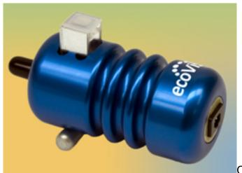
Ocean Optics has introduced the ecoVis, a compact, low-voltage light source (400 to 2,500 nm) with a built-in cuvette holder suitable for basic laboratory measurements. The light source has a rugged solid alloy housing that helps to dissipate heat and in-line fiber ports for absorbance and fluorescence measurements.
