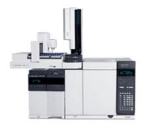
Agilent Technologies introduced the Agilent 5977A Series mass selective detector, which includes the benefits of the 7890B GC and features a redesigned inert mass spectrometer ion source that enhances performance with efficient ion collection.
