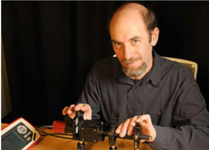
Using a low-cost apparatus designed to quickly and accurately measure the properties of handheld laser devices, National Institute of Standards and Technology (NIST) researchers tested 122 laser pointers and found that nearly 90% of green pointers and about 44% of red pointers tested were out of compliance with federal safety regulations. The NIST test apparatus was designed so that it can be replicated easily by other institutions.
