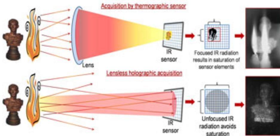
A team of Italian researchers has developed a new imaging technique that uses infrared (IR) digital holography to peer through chaotic conflagrations and capture potentially lifesaving and otherwise hidden details.
