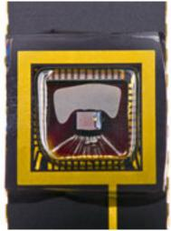
Organic sensors can be manufactured without the expensive post-processing step typically required for CMOS sensors, which involves for example applying micro-lenses to increase the amount of captured light. Every part of every single pixel, including the electronics, is sprayed with the liquid polymer solution, giving a surface that is 100% light-sensitive. The low noise and high frame rate properties of the organic sensors also make them a good fit for cameras.
