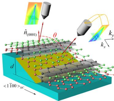
**click to enlarge** Diagram shows the experimental geometry of measuring graphene in silicon carbide trenches. The research showed a substantial electronic bandgap in the material.
